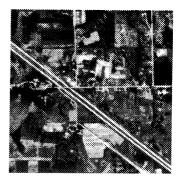
**Figure 2-57** TRANSPOSE has been used with this 512-by-512 aerial image to flip it diagonally (rotate it and create a mirror image).
